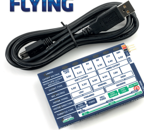
CC-010-0063-01 FIELD LINK programmer for FLYING
