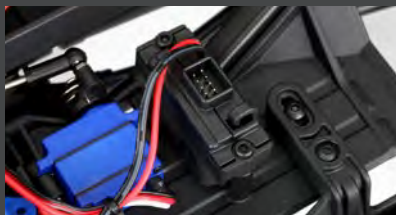
LED Lighting Module Installed
